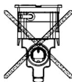
MULTICAL® 402 must not be mounted with the plastic box pointing upwards
