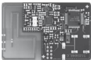
These radio modules are your first choice for reading via Kamstrup's hand-held reading systems, e.g. USB Meter Reader and hand-held terminal MT Pro, which operate in the licence-free frequency band in the 434 MHz area.
