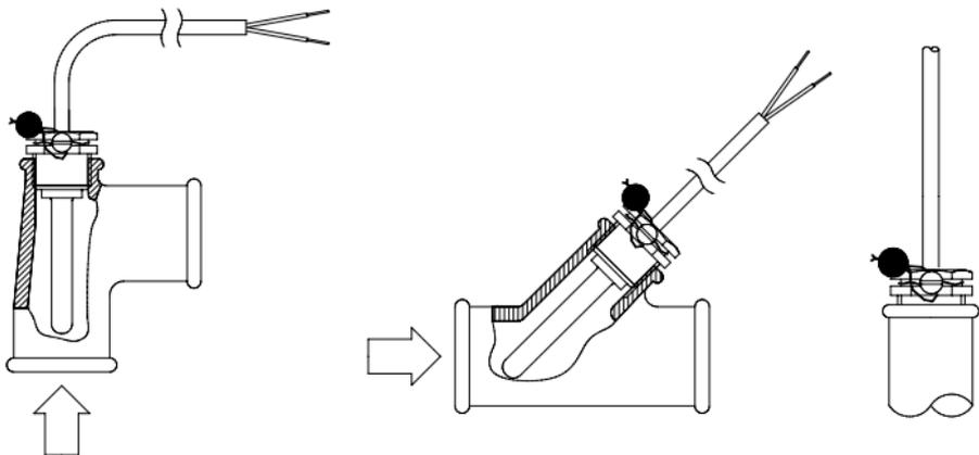
Temperature sensors should be inserted to the bottom of the pockets. If a short response time is required, “non-hardening” heat conducting paste can be used.
