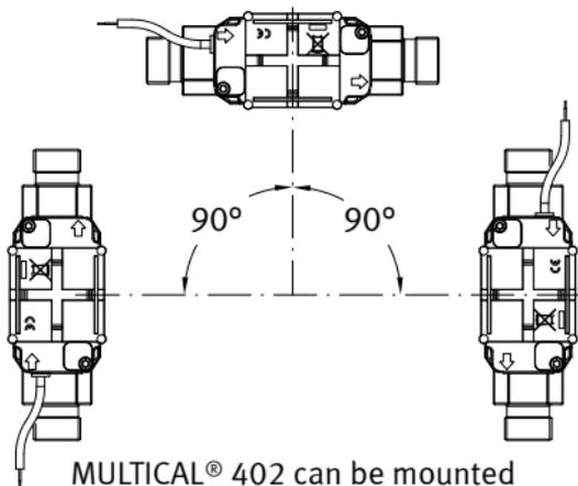
MULTICAL® 402 can be mounted vertically, horizontally or at an angle
