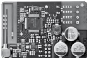
The radio module has been designed to form part of Kamstrup's hand-held Wireless M-Bus Reader system, which operates in the licence-free frequency band in the 868 MHz area.
