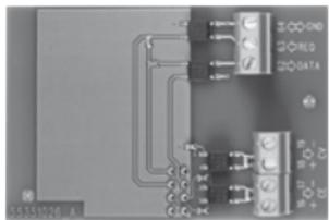
The data terminals are used for connection of e.g. a PC. The signal is passive and galvanically separated by means of optocouplers. Conversion into RS232 level requires connection of data cable 66-99-106 (D-Sub 9F) or 66-99-098 (USB) as follows:
