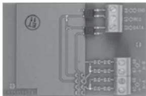
The data terminals are used for connection of e.g. a PC. The signal is passive and galvanically separated by means of optocouplers. Conversion into RS232 level requires connection of data cable 66-99-106 (D-Sub 9F) or 66-99-098 (USB) with the following connections:
