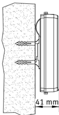
The wall fitting makes it possible to mount MULTICAL® 402 direct on an even wall. Use the fitting as a template for marking and drilling two 6 mm holes in the wall
