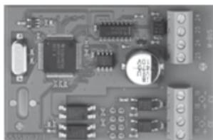
M-Bus module with primary, secondary and enhanced secondary addressing.
