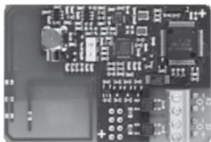
The radio modules have been optimized to form part of a Kamstrup radio network system, which operates in the licence-free frequency band in the 434 MHz area, but can also be used for the hand-held reading systems in the same frequency area.
