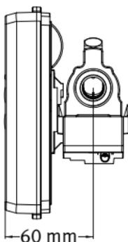
If minimum installation depth (G $\frac{3}{4}$  and G1) is required, the flow sensor is mounted with the plastic case pointing downwards and the calculator on the side
