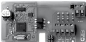
The M-Bus module 402029 comprises the same data packet as M-Bus module 6604 for MULTICAL® III/66-C and module 660S for MULTICAL® Compact/MULTICAL® 401.
