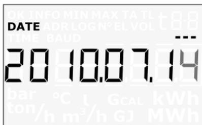
The value of the flashing digit can be changed by pressing the subkey
