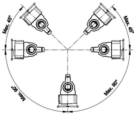
MULTICAL® 402 may be turned up to max. 45° and downwards for max. 90° in relation to the pipe axis.
